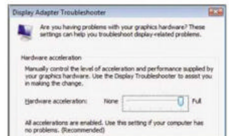
Use the display troubleshooter to check that hardware acceleration is on Full
