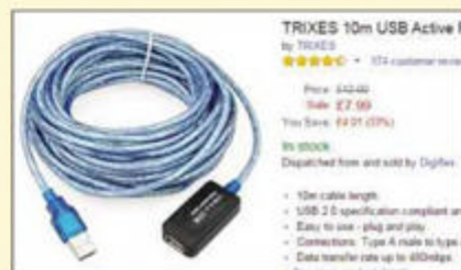
USB cables longer than 5m must be powered to maintain the signal strength
